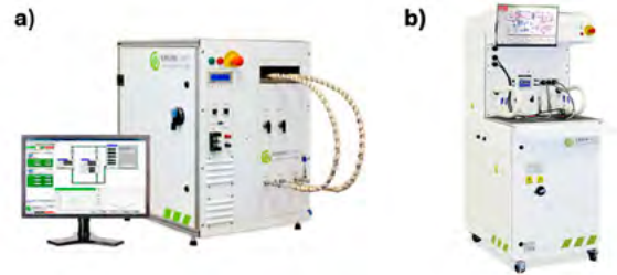
Figure 3: (a) Greenlight G40 PEM Fuel Cell Test Station and Greenlight E20 AEM Electrolyzer Test Station (b) Greenlight E40 PEM Electrolyzer Test Station.
