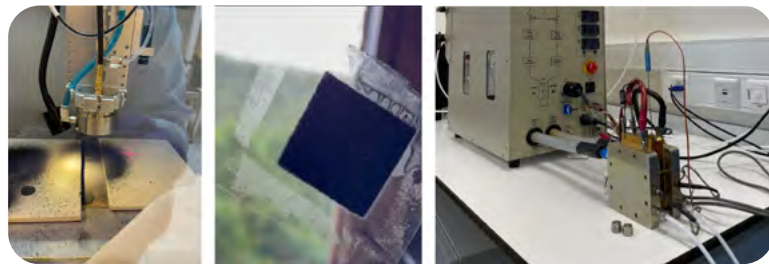
Figure 2: PEM fuel cell development process: coating of the catalyst layer, preparation of the membrane-electrode assembly (MEA), and single-cell test configuration.
